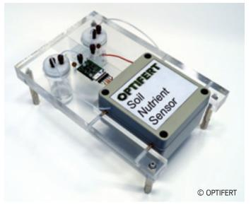
The analysis of all macronutrients NO3, NH4, K and PO4 is possible in a single run, within 120 seconds. Additionally, the sensor can be expanded to include a pollutant analysis by measuring further sample compounds like NO2 or Cl.
